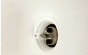
SPHERE INTERIOR SHOWING LAMP INSTALLED IN PORT
